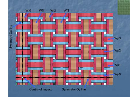
Notation of failing threads: Wpi(warps) and Wfi(wefts)
