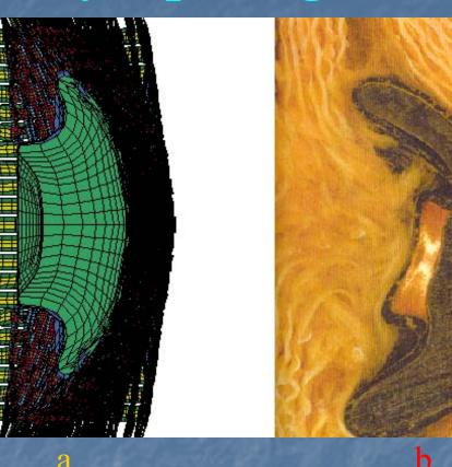
a - simulation result;b - experimental result (photo taken from the circular of TwaronCT textile)
