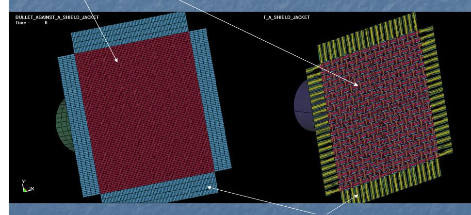
"Infinite" textile layer modeled by elastic supports
