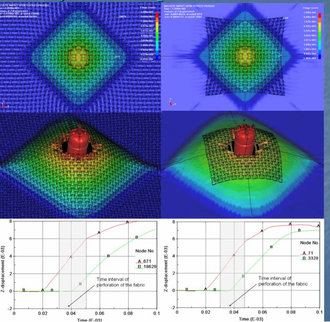
Propagation of the impact-excited transversal component of the wave across the tie boundary
