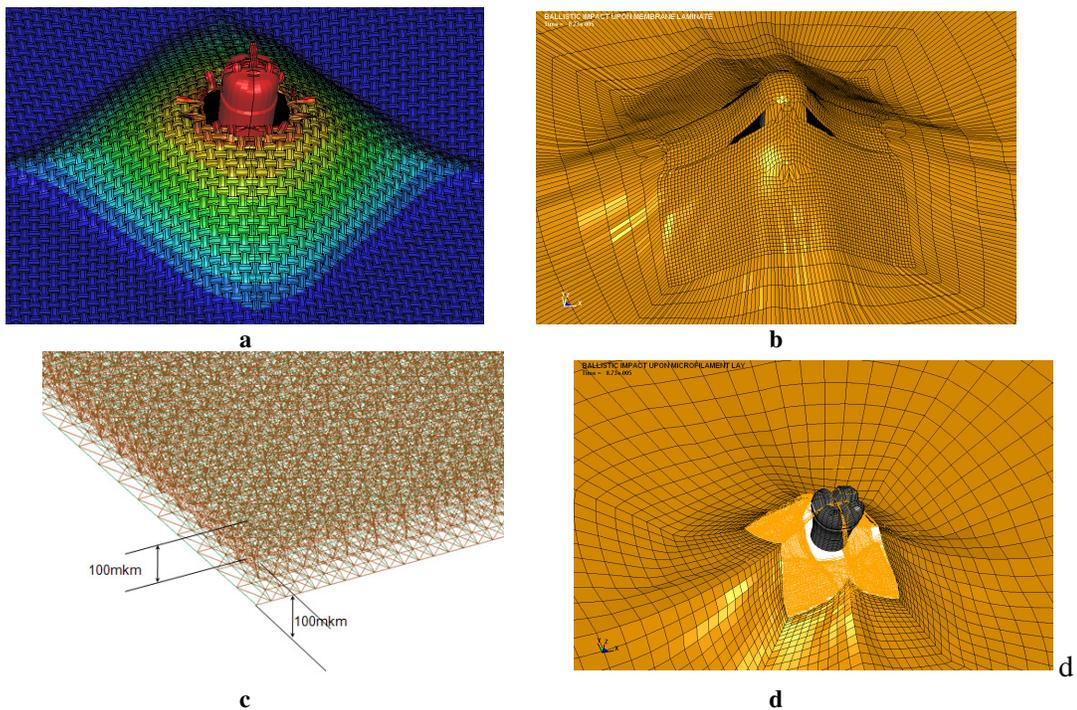
**Figure 2.** Finite element simulations of shooting through the woven textile structure (a), the orthotropic LTF model (b) and the mezzo-mechanical LTF model (c, d)
