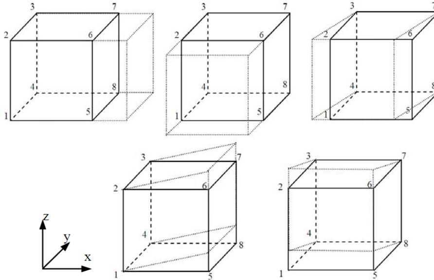
**Fig. 1.** Schemes for modeling pure stress in LS-DYNA
