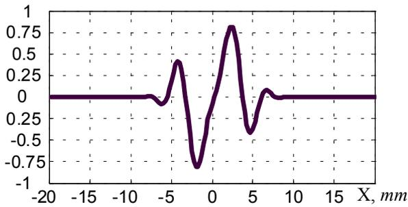
Figure 4: Distribution of relative acoustic pressure on the surface of the object
