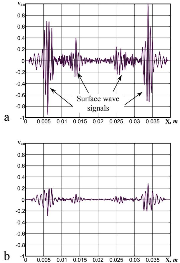
Figure 6: Distribution of particle velocity component  $v_y$  on the surface of the object (a) and 0.6mm below the surface (b) at time instance  $t=16.2\mu s$
