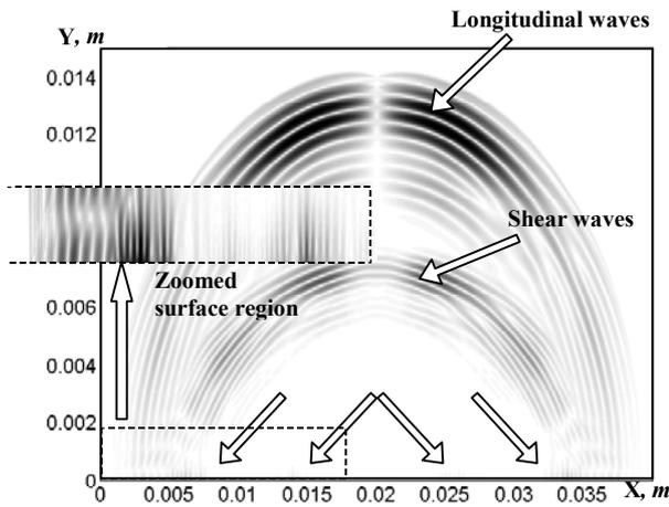
Figure 5: Distribution of modulus  $v = \sqrt{v_x + v_y}$  of particle velocity inside the object at time instance  $t=16.2\mu s$  after transmitter excitation.
