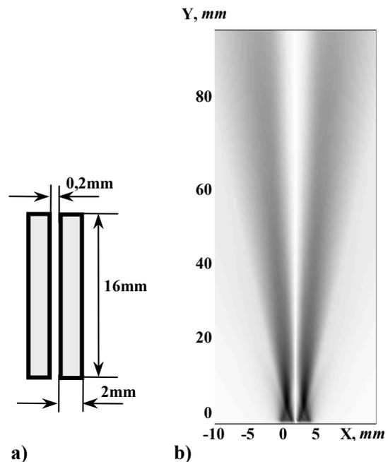
Figure 3: Dimensions of bipolar transducer (a) and structure of excited ultrasonic field
