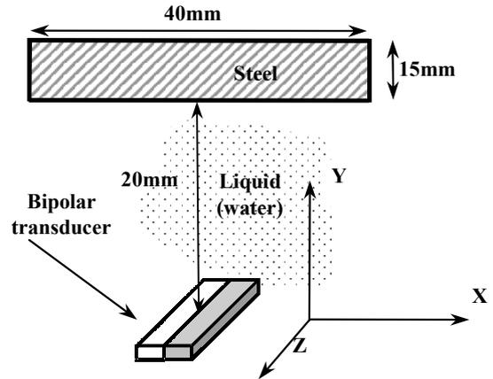
Figure 2: The geometry of simulated displacement measurement technique
