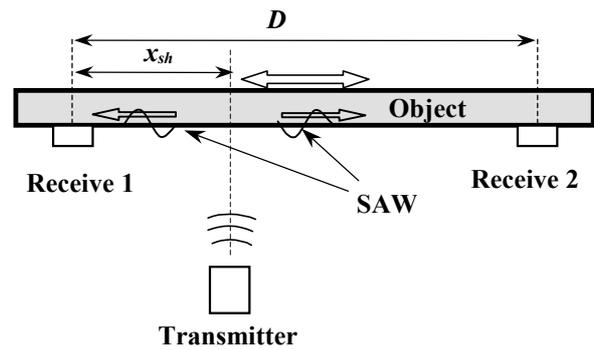
Figure 1: Displacement measurement technique using surface waves
